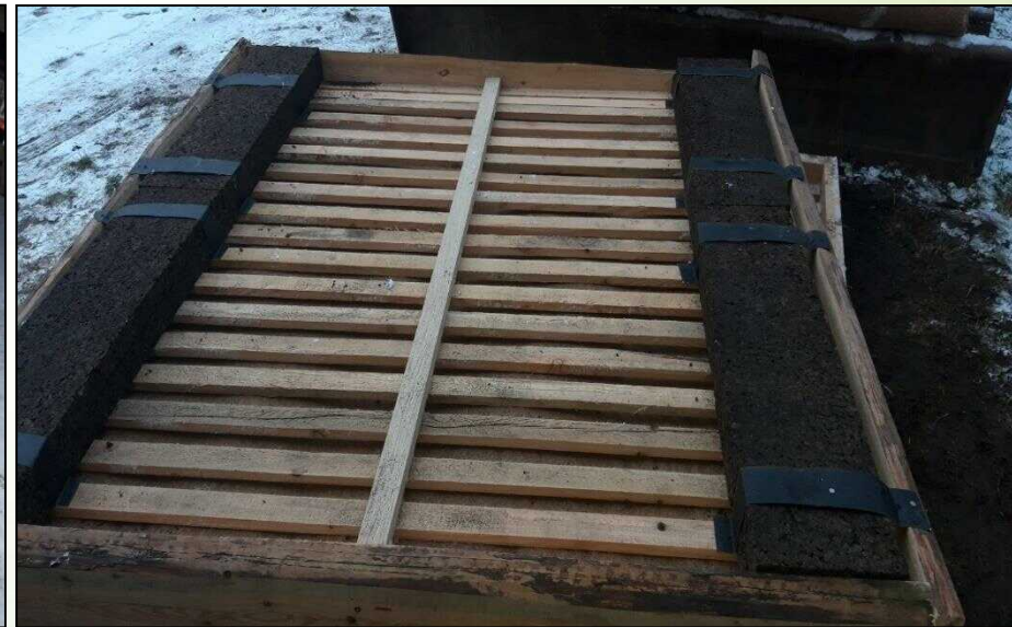
Floats made of expanded cork (W. Spychała)
