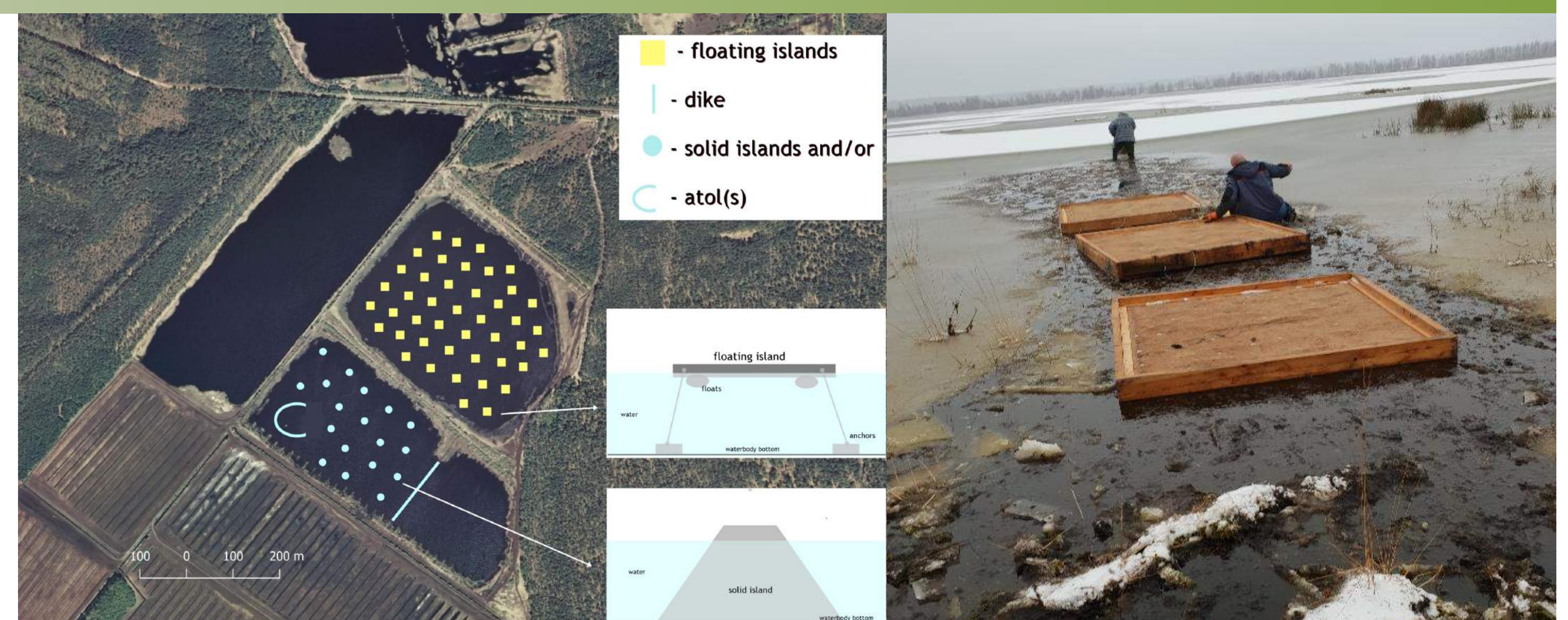
Technical planning for initializing overgrowing of water bodies; installing floating islands.
